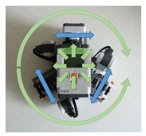
If we power all the wheels in the same direction, the platform would simply rotate about its centre. However, it is possible to make the platform move in useful directions too.
