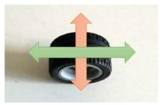
Omniwheels, being able to move freely in one direction and retain grip in the other can be mounted in a triangular fashion. When these wheels are mounted at 120° angles, they make a very stable platform. This type of setup is also known as a Killough platform.
